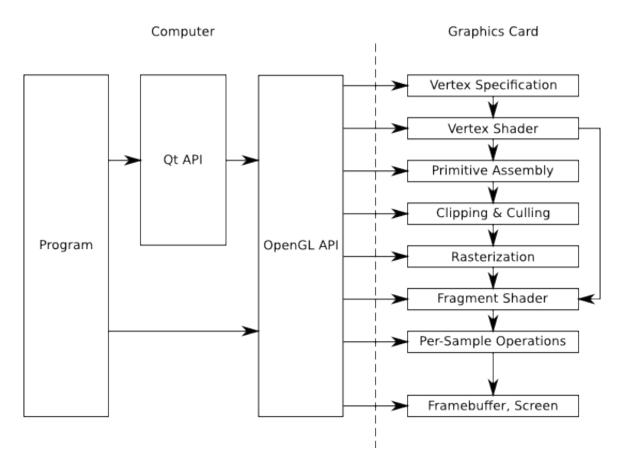
The graphics card has its own memory and a GPU just like a small powerful computer that is highly specialized in processing 3D data. Programs that run on the GPU are called shaders. Both the host computer and the graphics card can work independently, and you should keep both of them busy at the same time to take full advantage of hardware acceleration.
